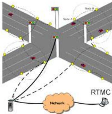
The WSN-based traffic information collecting system is comprised of wireless traffic information collection nodes (TICoN), wireless data aggregation node (DAN) and remote traffic monitoring center (RTMC). TICoN nodes collect and process real-time information in a distributed and coordinated fashion. They transmit the results to the DAN node wirelessly. Then, the DAN node transfers the information to the RTMC or uses the information to control the traffic light.
